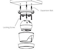
Fix the pedestal by drilling locking holes around the sticker and inserting three expansion bolts into the holes and fastening it with three locking screws.
