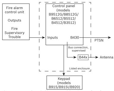
Figure 1.13: Control panel with a B44x module and a B430 (PSTN) module
