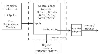
Figure 1.6: Control panel with on-board IP
