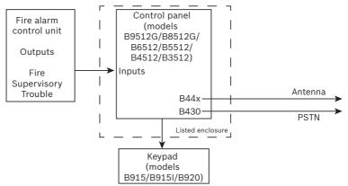
Figure 1.12: Control panel with a compatible cellular module and a 430 (PSTN) module
