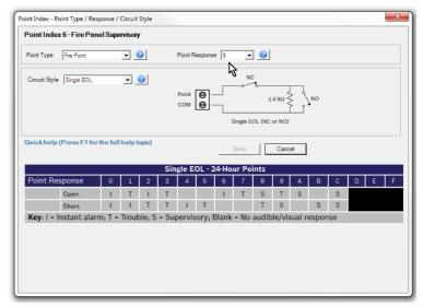
Figure 1.19: Point Type Response and Circuit Style
