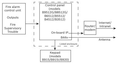
Figure 1.11: Control panel with on-board IP and a B44x (cellular) module
