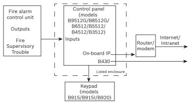
Figure 1.8: Control panel with on-board IP and a 430 (PSTN) module NOTES: The B9512G-E/B8512G-E/B5512E/B4512E/B3512E control panels do not include on-board IP.
