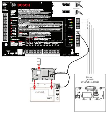
Figure 1.14: B9512G/B8512G\* control panel with a B44x (cellular) module connected through a B450 module
