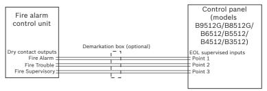
Figure 1.1: Fire alarm control unit dry contact outputs to control panel points 1, 2, and 3
