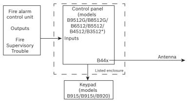
Figure 1.10: Control panel\* with a B44x (cellular) module
