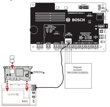
Figure 1.15: B6512/B5512/B4512/B3512\* control panel with a B44x (cellular) module connected through a B450 module
