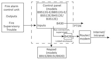
Figure 1.9: Control panel with a B426 module and a B430 (PSTN) module NOTES: The B9512G-E/B8512G-E/B5512E/B4512E/B3512E control panels require a B426 for IP.
