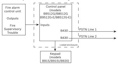
Figure 1.5: Control panel with 2 B430 (PSTN) modules
