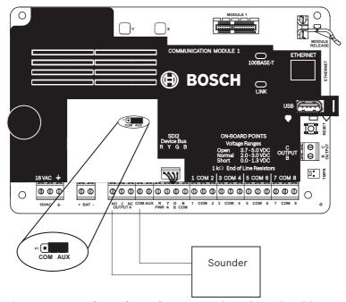
Figure 1.16: B6512/B5512/B4512/B3512 control panel sounder wiring and hardware configuration
