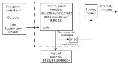
Figure 1.7: Control panel with a B426 module
