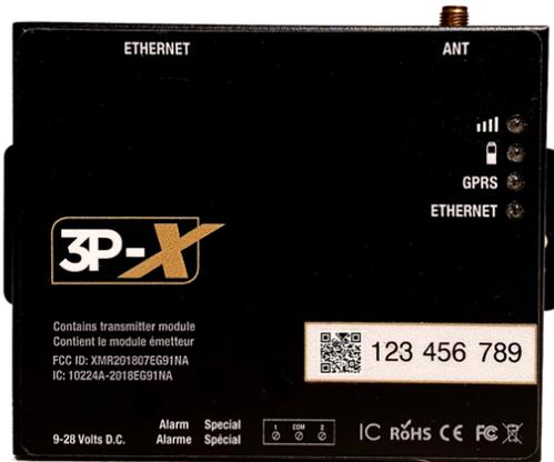
Check the Cellular Signal Bars to ensure you have a connection to the local cellular network.
